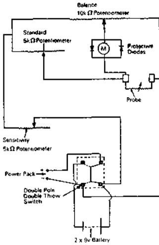
Figure 3 Circuit diagram for the environmental comparator.
