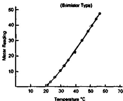
Figure 8 Calibration curve for the temperature sensitive probe.
