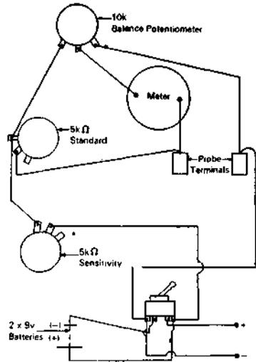
Figure 4 Wiring aid for environmental comparator.
