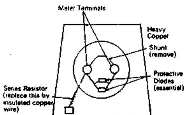
Figure 1 Diagram showing shunt and protective diodes of meter viewed from below.
