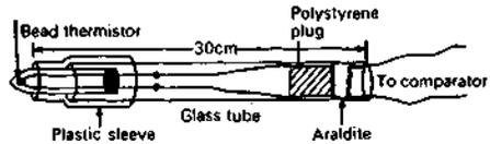
Figure 6 Bead thermistor temperature sensitive probe.
