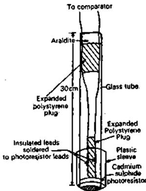
Figure 5 Light sensitive probe.
