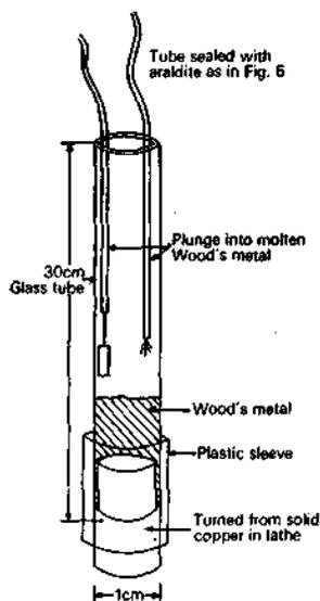
Figure 7 Brimistor temperature sensitive probe.
